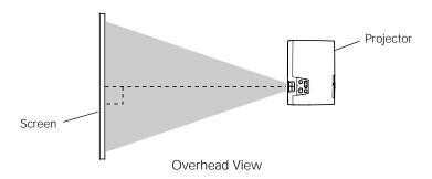
It's best to place the projector level with the bottom of the screen, or slightly lower. If you place the projector below screen level, you'll have to tilt it up by extending its feet. This causes the image to lose its square shape, but the projector automatically compensates. You can further correct the distortion by pressing the Keystone button as described on page 19.
