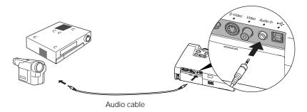
Connect the other end of the cable to the audio-output connector on your video equipment. You may need to use an adapter to plug in the cable.
