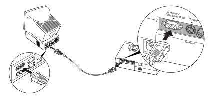
3. Tighten the screws on the connectors.
