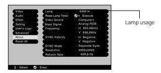
The life span of the lamp is about 1500 hours. If the number shown is close to 1500, make sure you have a spare lamp handy.
