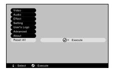
Select Reset All and press the Enter button on the remote control to display the confirmation screen. Select Yes to reset all the default settings or No to cancel.
