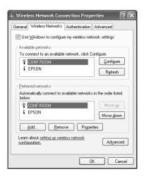
13. Verify that you've enabled your computer's connection to the access point. It should be listed as shown above, with the small con next to it, indicating a connection.
