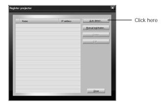
3. Click Auto detect to locate projectors currently operating on the network. Or click Manual registration and enter the projector's name and network address.
