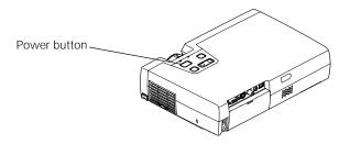
The  $\circ$  power light flashes green as the projector warms up, and the projection lamp comes on in about 40 seconds.
